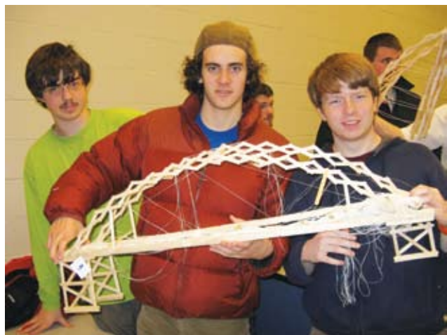
U-32 entered two strong teams in Norwich University's annual bridge truss competition. RB Johnson, Jordan Black-Deegan, and Dan Thompson's bridge weighed less than one pound and held over 60 lbs. before breaking!
